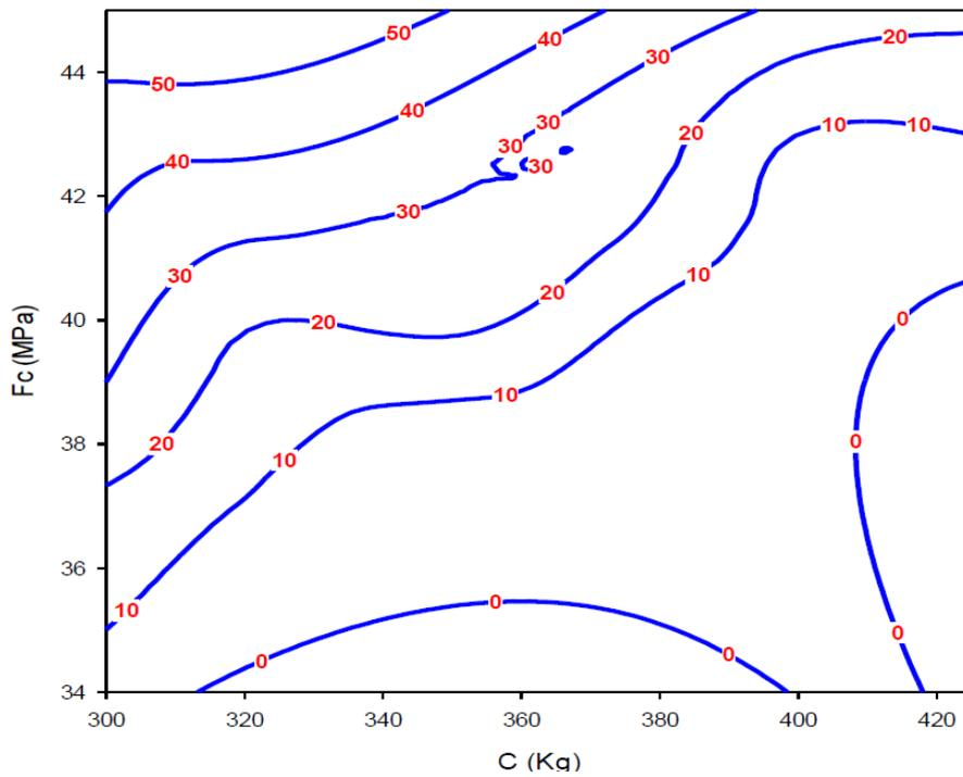
Figure 5. Contour of micro silica (Kg) with  $F_c$  (MPa) vs. Cement (Kg) value from Eq. (11)
