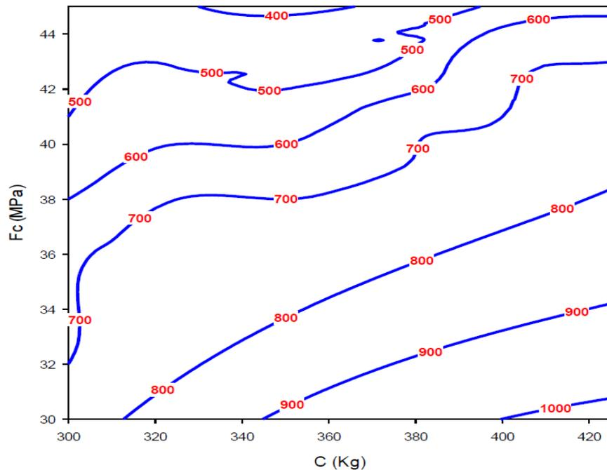
Figure 3. Contour of fine aggregate with  $F_c$  (MPa) vs. Cement (Kg) value from Eq. (11)
