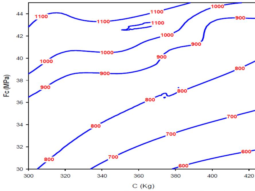
Figure 4. Contour of coarse aggregate with  $F_c$  (MPa) vs. Cement (Kg) value from Eq. (11)
