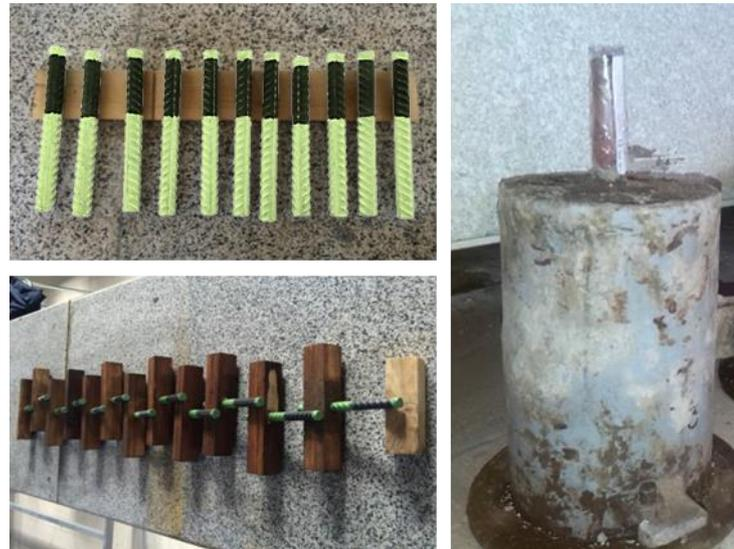
Fig. 1. Preparing of Pullout Specimens.
