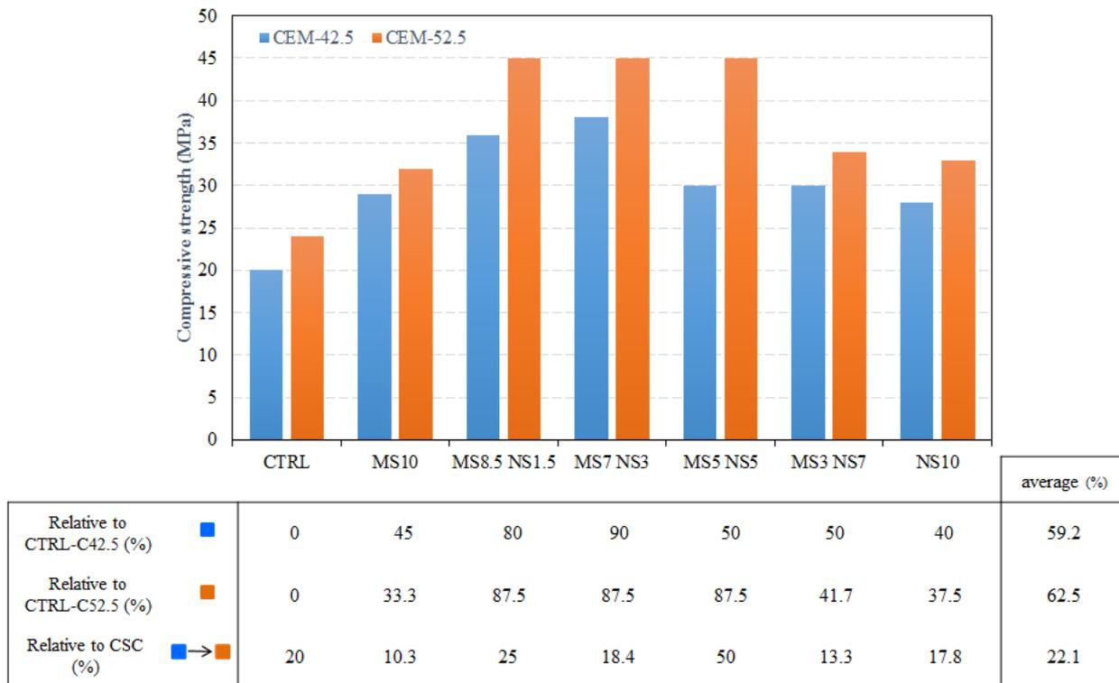
**Fig.2.** Compressive strength of specimens containing different percentages of MS and NS.
