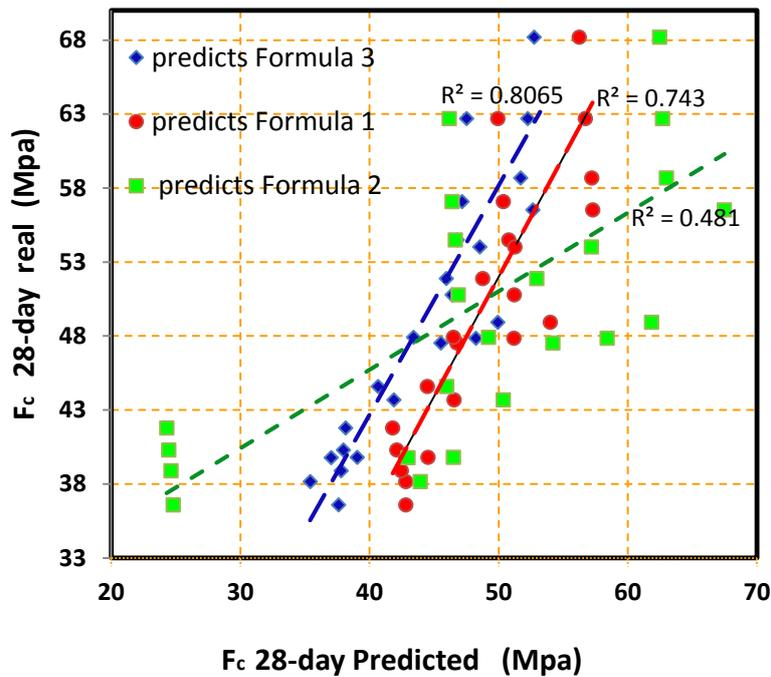
Fig1. Prediction of Ferro-cement mortar by suggestion fourmula 1
