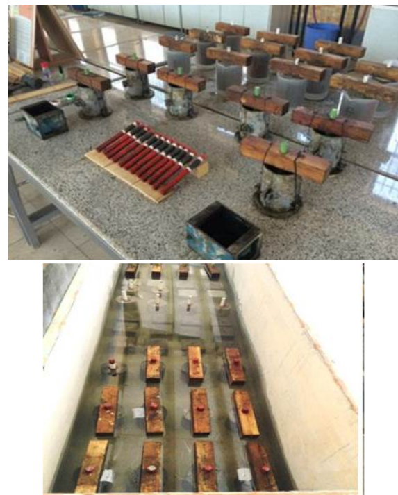
Fig. 2. Representation of the construction and curing process of the cylindrical specimens.
