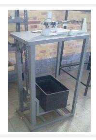
Name: Sand Equivalent Value of Soils and Fine Aggregate
