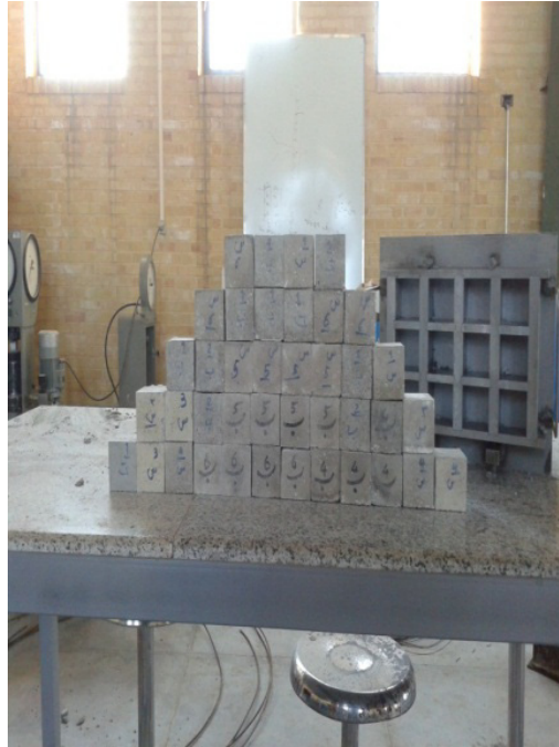
Fig. 2. Specimens sample of compressive strength test.
